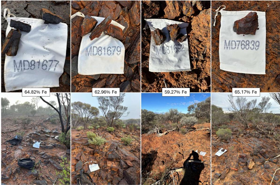
*Figure 10. Example rock-chip sample and outcrop photos.*
