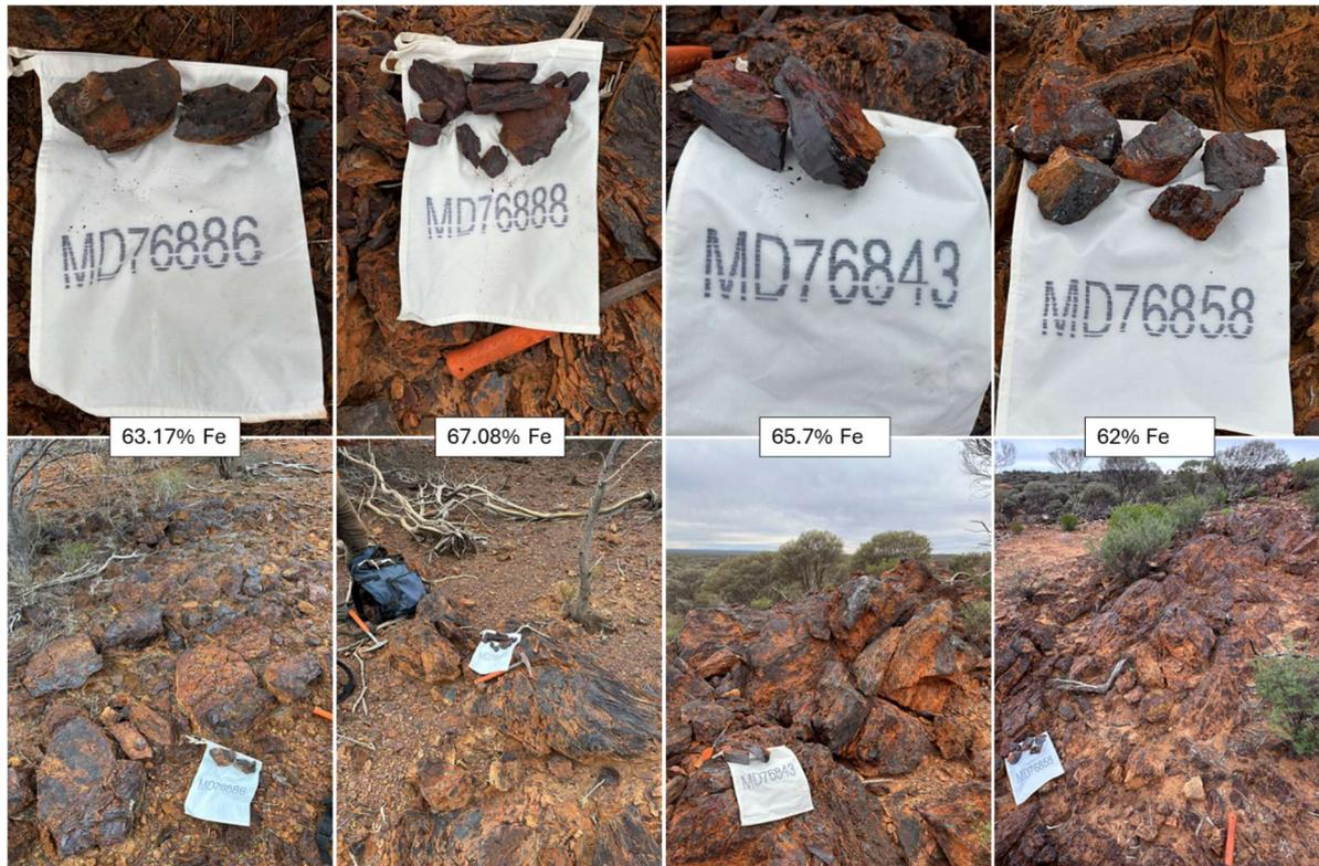
*Figure 11. Example rock-chip sample and outcrop photos.*
