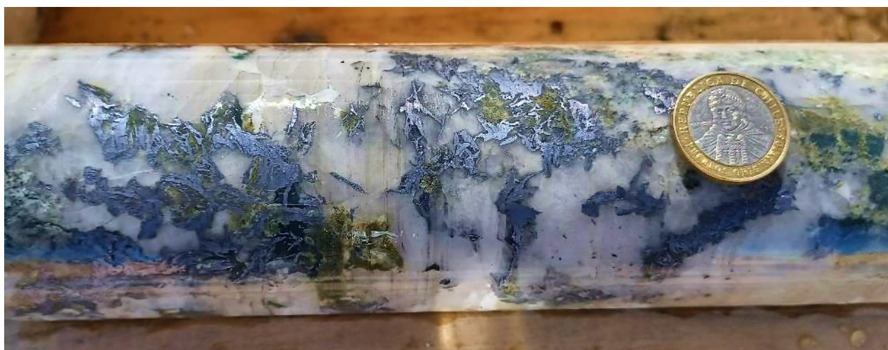
Figure 6: Example of high-grade molybdenum mineralisation in hole CMLCD014, 4,350ppm Mo (1.70% CuEq) (498m to 500m). 3
