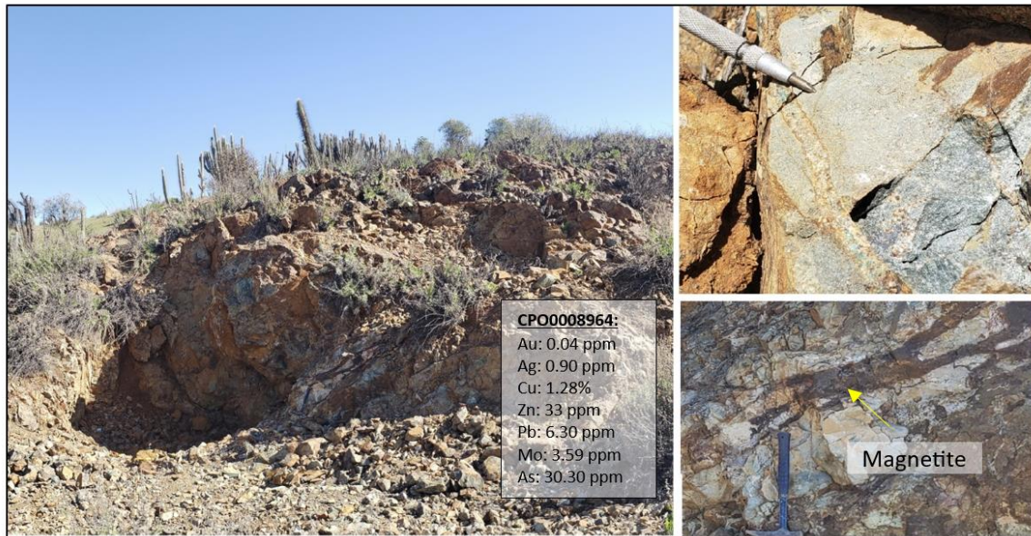
Figure 9: Sample CPO0008964 - Andesite host rock, brecciated texture with chlorite-epidote-albite alteration, featuring mineralisation in vugs and patchy zones with limonite, copper oxide, and magnetite 17 .
