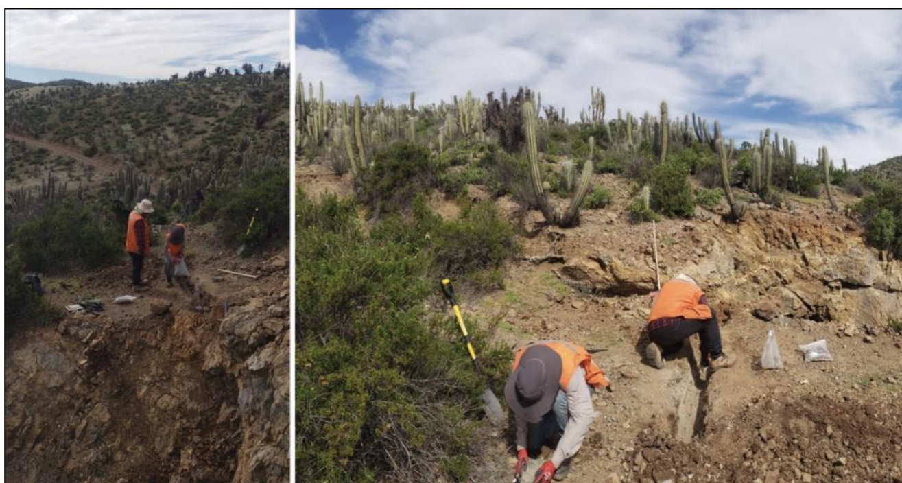
Figure 12: Trenching at an andesite outcrop with silica-albite-sericite alteration within a silicified and brecciated structure. Mineralisation shown to consist of quartz, iron oxides, and copper oxides. Samples CPO0009117-CPO0009118- CPO0009119 Trench 1 (5.5m at 0.88% CuEq) 18 .
