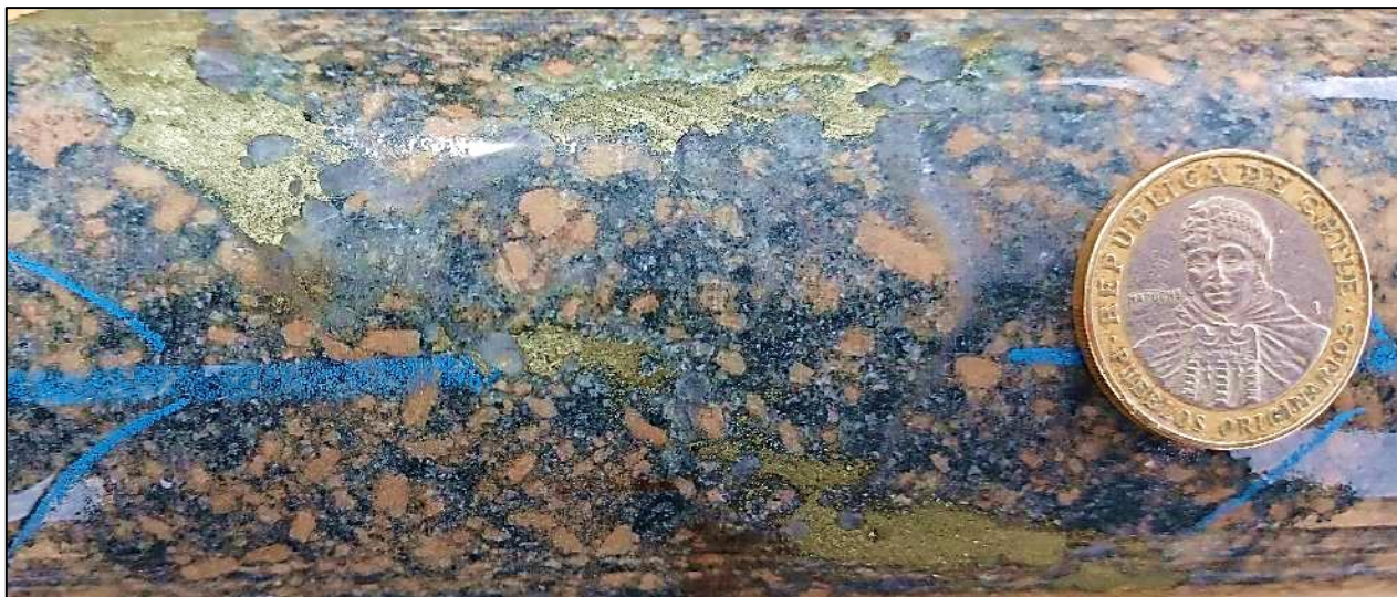
Figure 5: Example of high-grade copper mineralisation in hole CMLCD014, 1.74% CuEq (416m to 418m). 3
