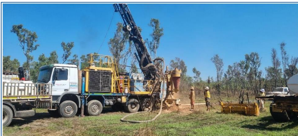
Figure 2: Aircore drilling in the field at EverGreen’s EL 31774
