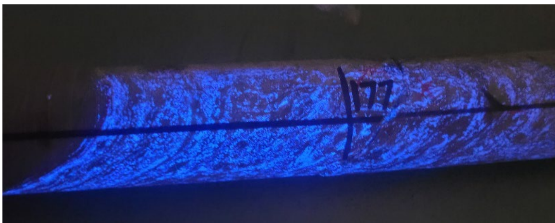
Figure 5 – WQDD013 (0.65m @ 18.35 WO 3 ) scheelite intersection under UV light
