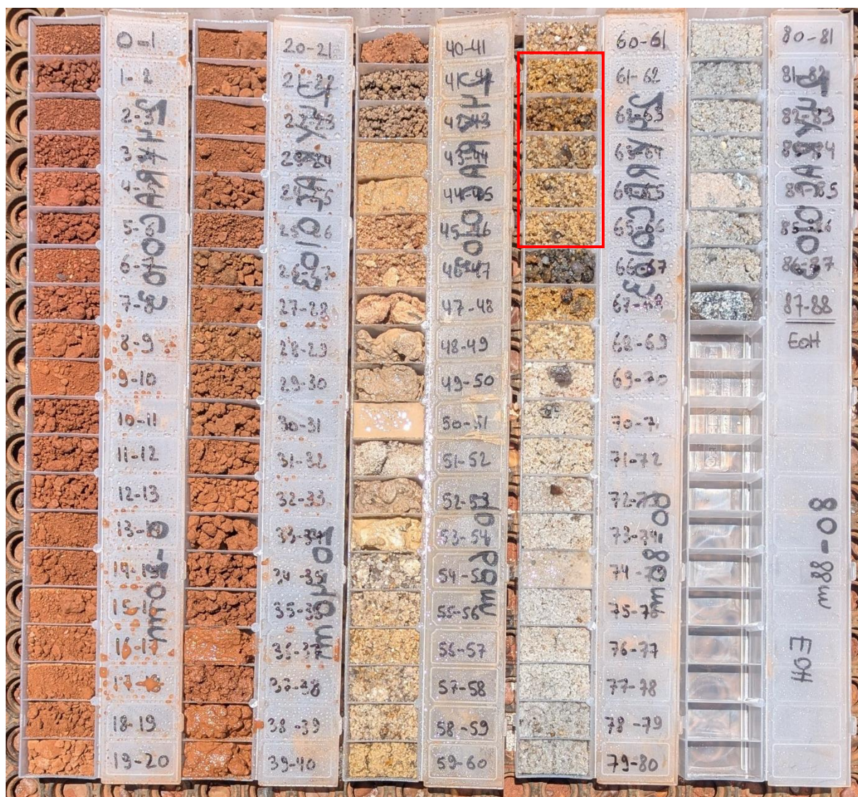
Figure 5. 24YRAC103 Chip trays. Note the mineralised zone (highlighted in red) developed above the reduced carbonaceous sand interval (66-67m).
