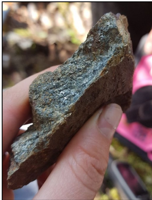
Figure 3: Photo of the mineralised sample 1292094 from Vein #2 at the Flicka Zone, which assayed at 19.4ppm (19.4 g/t Au)
