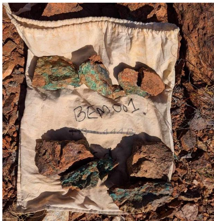
Figure 1: Photo of rock chip BEM001 showing secondary copper oxides and carbonates coating an iron rich gossan. BEM001 returned assay of 6.6% Cu, 0.7% Pb, 5.1g/t Ag, 0.1g/t Au.
