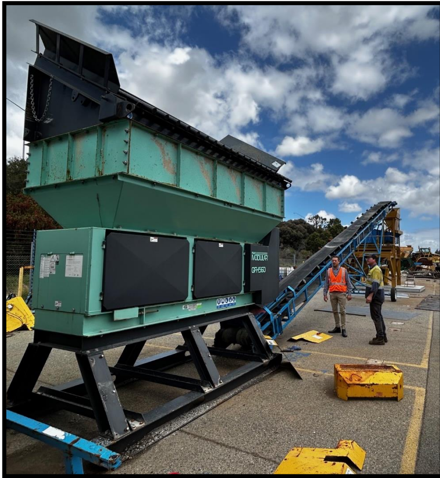
Figure 2: Feeder circuit of Gekko processing plant
