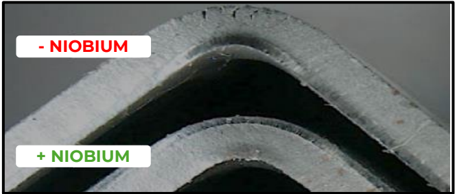
IMPROVED FLAT SHEET FORMABILITY WITH NIObIUM 3
