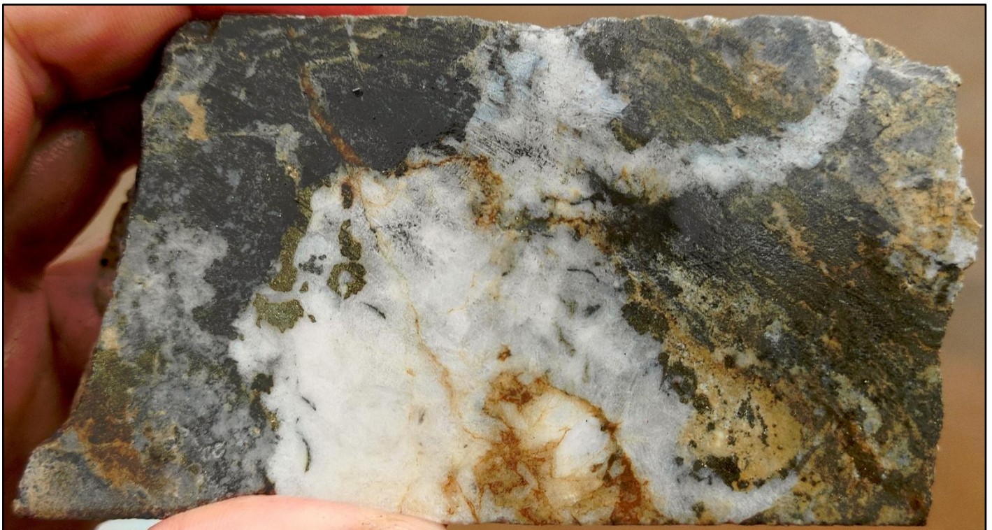
Figure 6. Gold-only mineralisation associated with quartz-carbonate veining in endoskarn from 595.5m downhole depth in ZRSD24163 – 5.3g/t Au.
