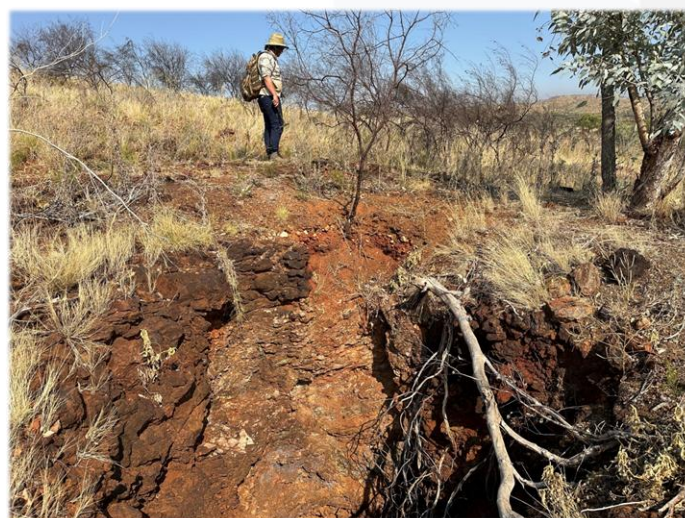
Figure 4. Pronuba western zone historical workings showing copper oxide mineralisation including malachite and iron oxides. Mullock sampling recorded assays of 5.7% Cu and pXRF readings of 10.6% Cu.
