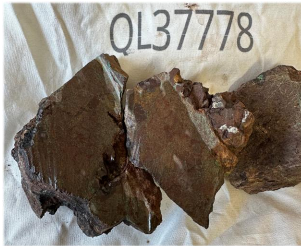
Figure 3. Pronuba east zone sub-cropping high grade massive copper oxide gossan mineralisation from rock chip sample QL37778 with pXRF readings of 30.4%, 31.8%, 41.6% and 36.2% Cu.
