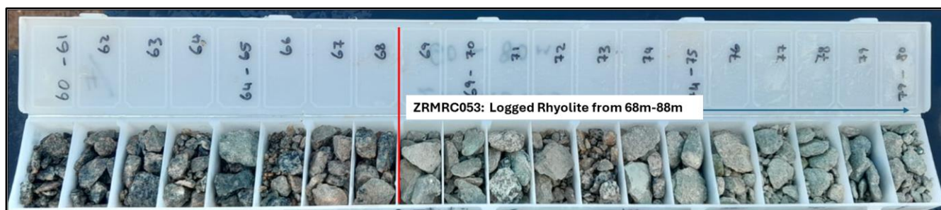
Figure 5: Image of RC chips from the first drill hole of the new campaign at Red Mountain (ZRMDD053); logged rhyolite from 68-88 (true width ~10m) -assays pending at time of writing
