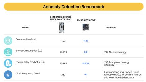
Table 2: Anomaly Detection Benchmark compared to STMicroelectronics NUCLEO-H7A3ZI-Q.
