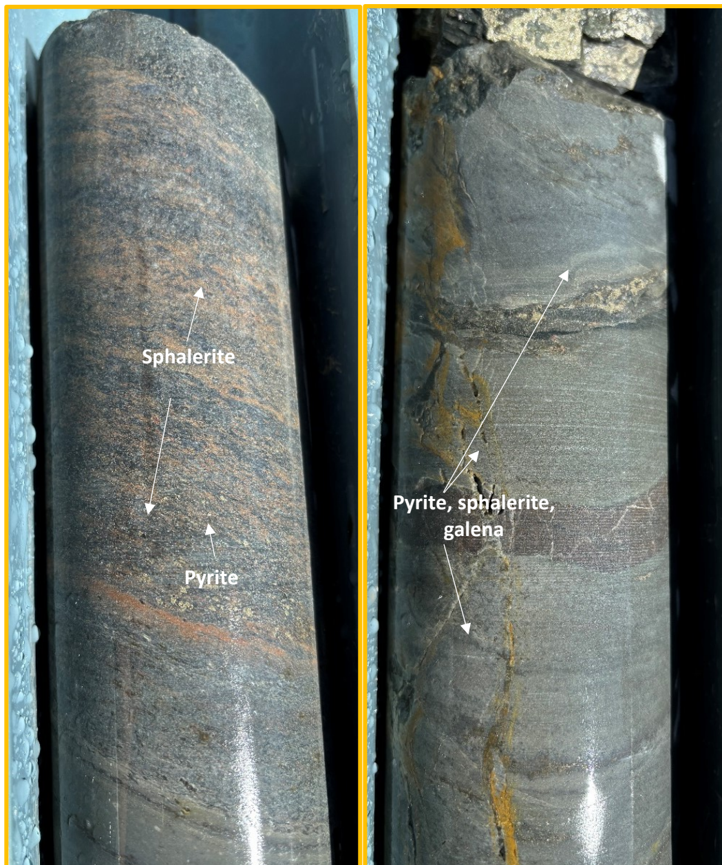
Figure 6: Hanging wall rocks in A3DD004 with low grade sulphides along bedding. Left: 107-108m grading 1.1g/t Au, 68g/t Ag & 1.3% Pb+Zn Right: 109-110m grading 0.5g/t Au & 42g/t Ag.
