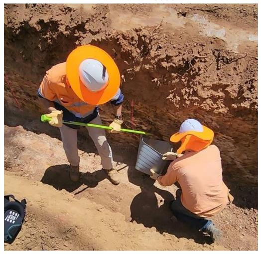
Figure 6: Banshee channel sampling along lower walls of shallow historical trenches
