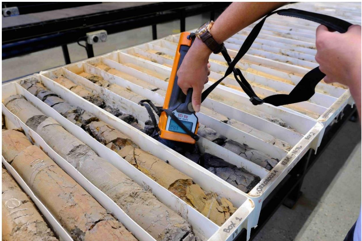
Figure 2: Spectrometer 153 cps Orroroo 2A reduced sediment margin.
