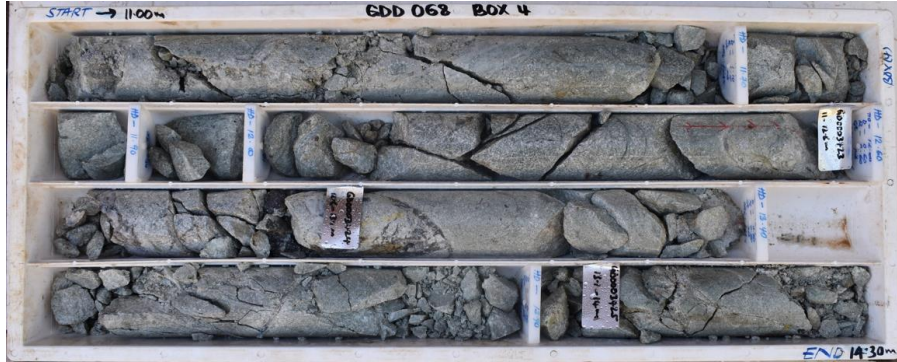
GDD068 Se-Cly-Py Alt. Dr. Po + CBM Veins (yellow sphalerite) (10.2m @ 3.65g/t Au from 10m)
