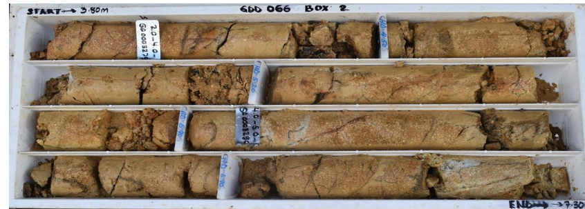
GDD066 Oxide. Dr.Po. Mn Oxide fractures (after Sph-Gal) (6m @ 2.46g/t Au from 4 - 10m)
