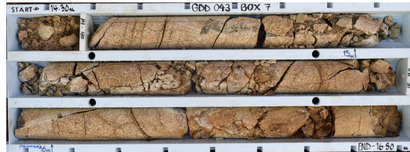
GDD043 Abi-Kila Oxide Dr.Po. Remmenant CBM and sulphide veins (23.6m @ 2.91g/t Au from 7.4m, including 13.5m @ 4.60g/t Au from 17.5m)
