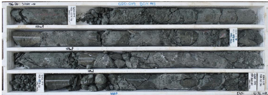
GDD014 Brecciated meta basalt post CBM veining
