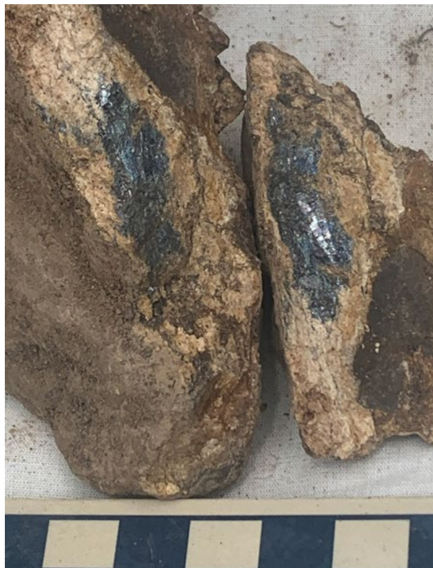
Figure 4: Sample MVS17: Vein of white and minor pale green antimony oxide (antimony trioxide \text{Sb}_2\text{O}_3 , 55%) and portions with silvery-grey antimony sulphide (stibnite, \text{Sb}_2\text{S}_3 , 10%) up to 32mmx12mm, hosted in grey, silicified pelite (35%). Note the acicular (elongate) stibnite crystals. Single rock collected from mine dump (GDA94, 56J, 6614288mN, 400905mE) and fragmented for examination (scale bar: Centimetre divisions). Sample dispatched for assay and results anticipated in 2-3 weeks.
