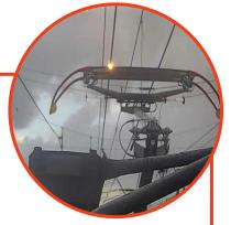
Real time detection of excessive arcing is a part of the OHCAM software modules. The system detects unusual arcing and sparking events which assists with condition monitoring of the pantograph carbon and overhead line geometry.
