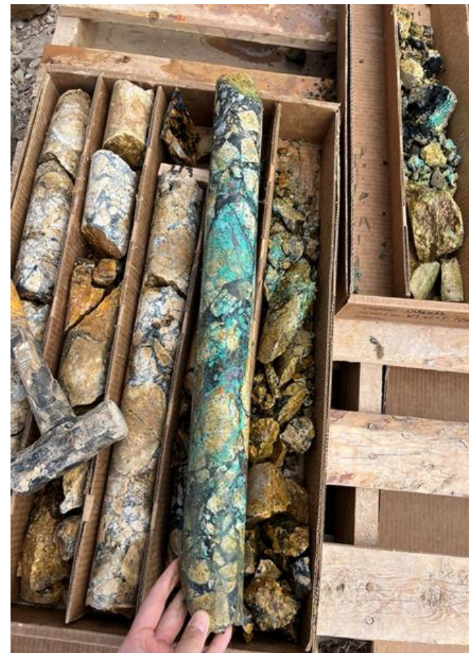
Copper mineralisation at 14-16m down NY2024-DDH2 which assayed 3.25% Cu, New Years prospect
