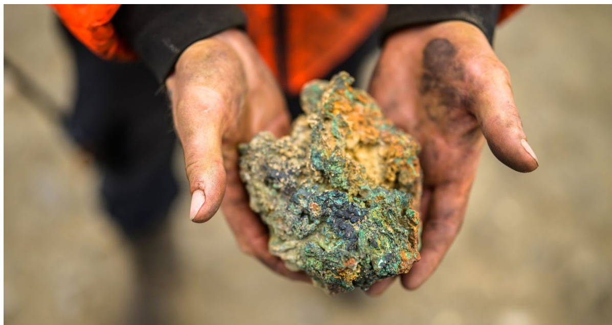
Figure 1: Copper gossan from the Hailstorm Prospect. This is massive chalcocite (copper sulphide) and returned a laboratory assay grade of >50% Cu (50% is the upper limit of the assay technique used).
