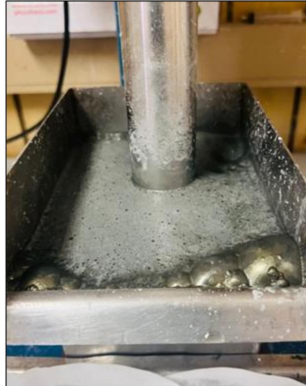
Typical Flotation test producing Rougher concentrate
