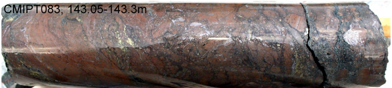
Figure 5. Hole CMIPT083: high-grade massive and brecciated massive sphalerite (red-brown) with lesser galena. Up to 3% chalcopyrite (yellow) is present in places.
