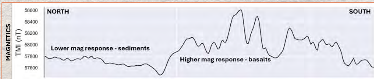
Profile of total magnetic intensity along line 7740 (N/S) through the basalt-sediment contact within Hulk sub basin target
