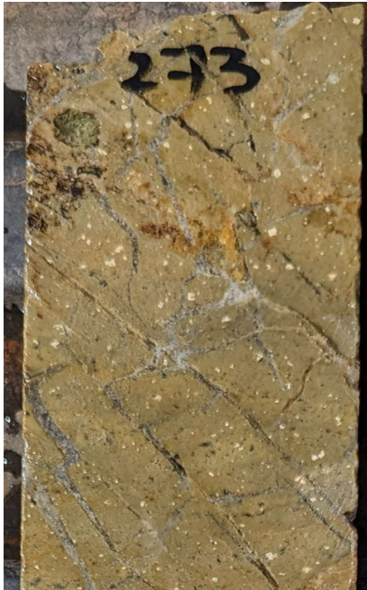
Gold Mineralisation (25.3 g/t Au) in Rhyolite at 272.3-273 m in LRCD152 (HQ Core) 1
