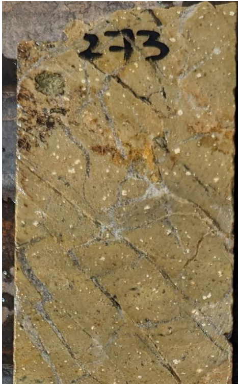
Gold Mineralisation (25.3 g/t Au) in Rhyolite at 272.3-273 m in LRCD152 (HQ Core) 1
