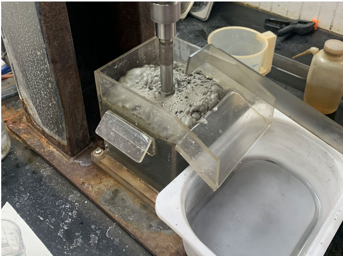
Figure 4. Flotation testing of Dolomicrite master composite at Auralia Metallurgy
