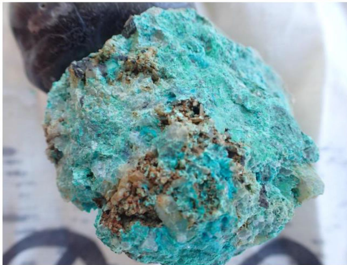
Sample ESS02045 – A white, frothy to glassy quartz vein hosting abundant drusy cavities lined with euhedral prismatic quartz crystals with supergene malachite and chrysocolla developed over sooty tenorite
