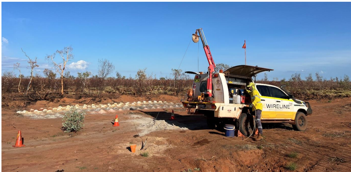
Figure 1. Wireline Service Group undertaking down-hole televIEWer surveying at drill-hole 24XCRC097.
