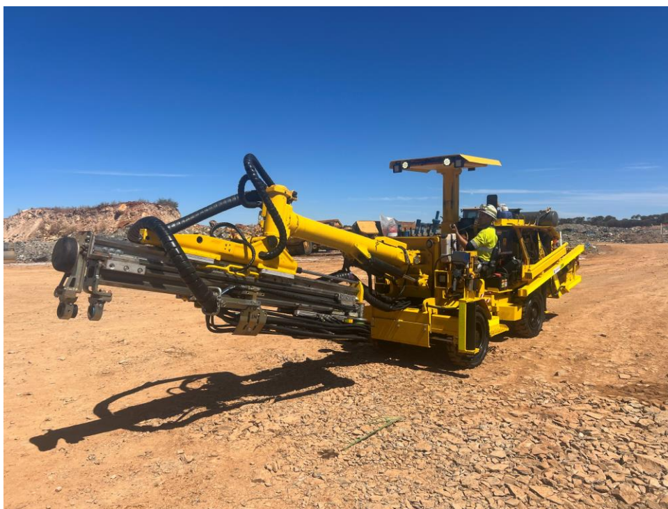
Figure 1 – Zero hour rebuild Atlas H104 development drill arriving at Second Fortune
