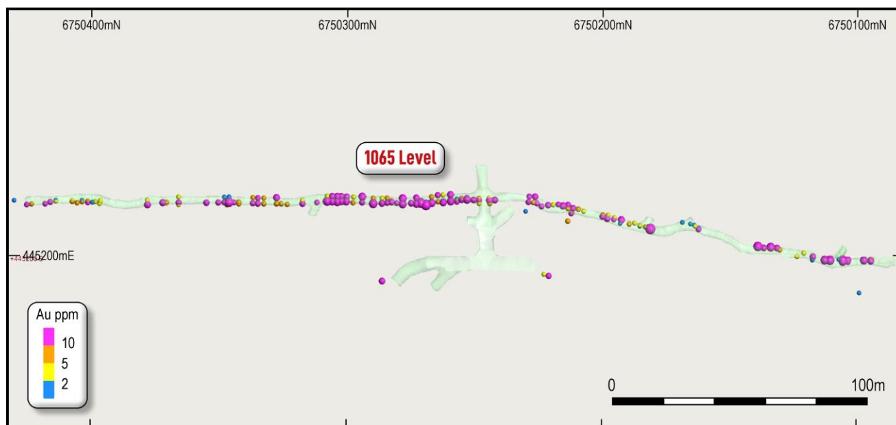
Figure 5 – Ore drive development face sampling on the 1065 Level
