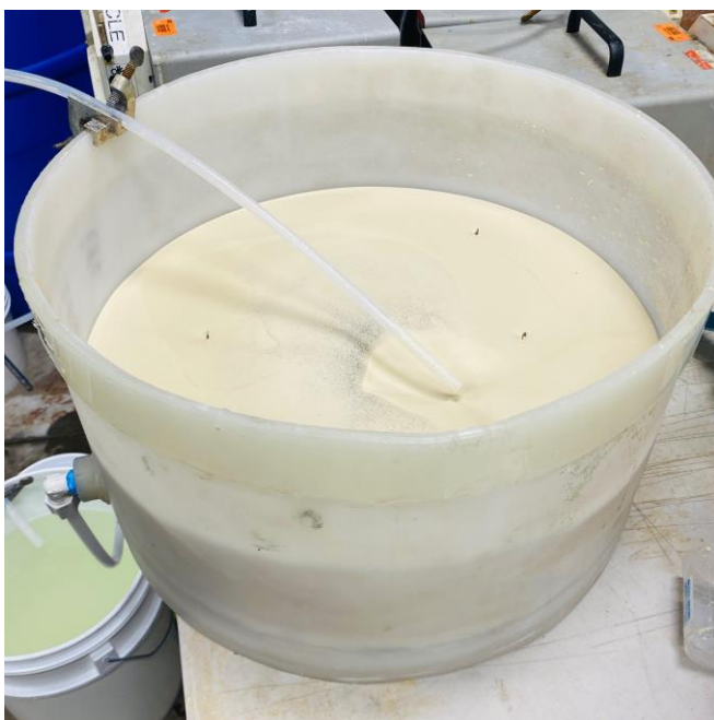
Figure 4: Filtering stage and resultant filter cake post water-leaching and impurity removal.
