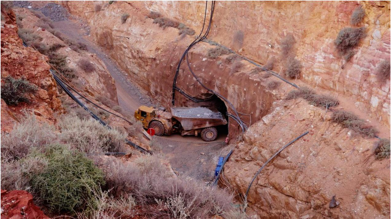
*Figure 2 - Underground haul truck emerging from Second Fortune decline*
