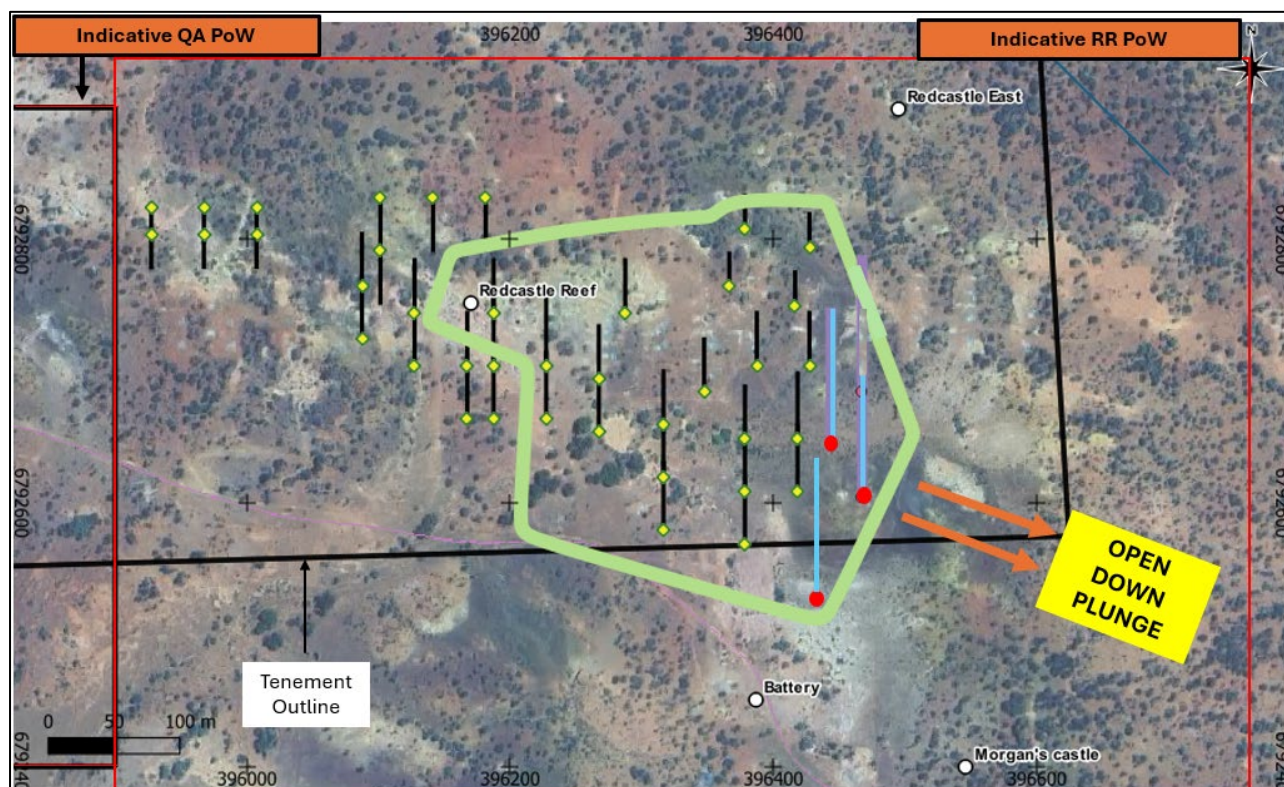
FIGURE 5 - Planned drilling at Redcastle Reef with deep holes shown in blue (plan view)
