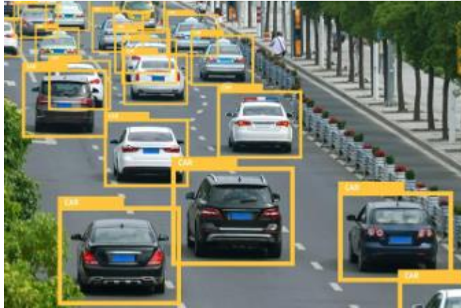
Figure 2: Example of Bounding Boxes used in the context of Vehicle Detection
