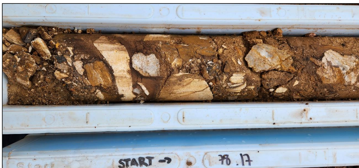
MLJDD020_178.0m_Polymictic Breccia with silica-pyrite clast
