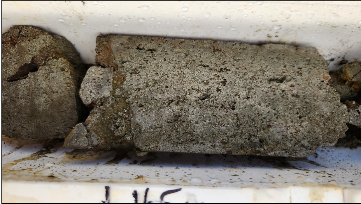
MLJDD018_164.5m_Massive pyrite in Breccia
