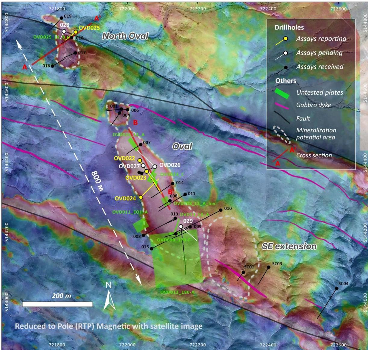
Figure 1. Plan view of drillhole locations on high resolution magnetic map (RTP)
