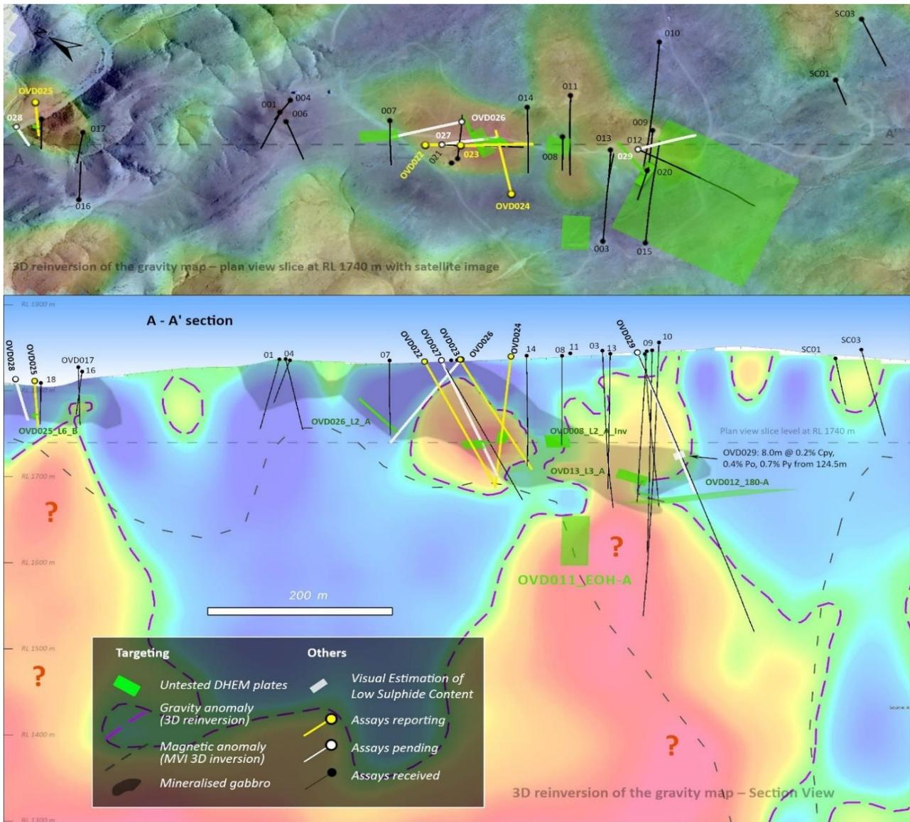
Figure 4: Long Section, Phase 2 drilling untested DHEM survey plates on Inverted Gravity Background<sup>9</sup>
