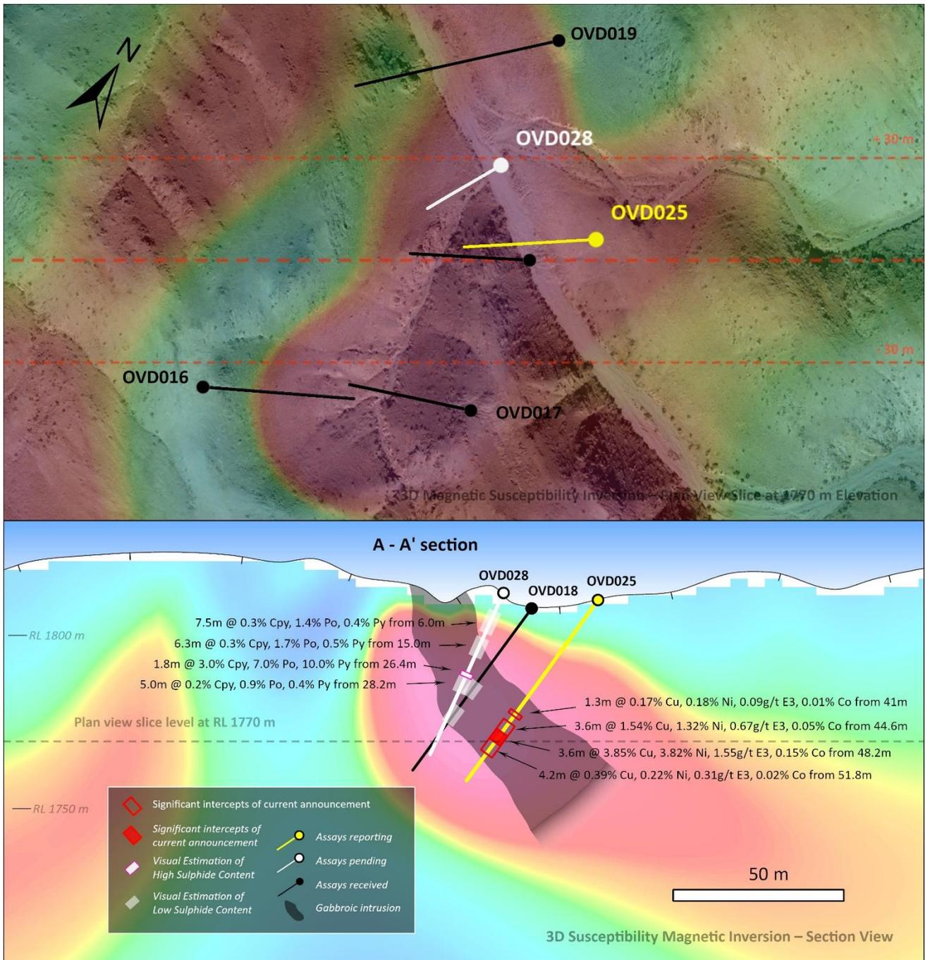
Figure 2: Typical Section, OVD025 and OVD028<sup>8</sup> results, Interpreted Mineralisation on Inverted Magnetics Background
