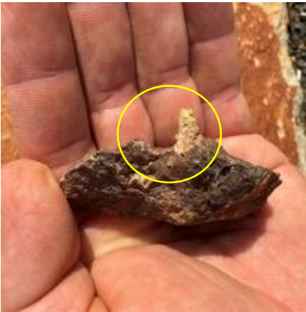
Visible gold in iron oxide vein located at Sing Six prospect
