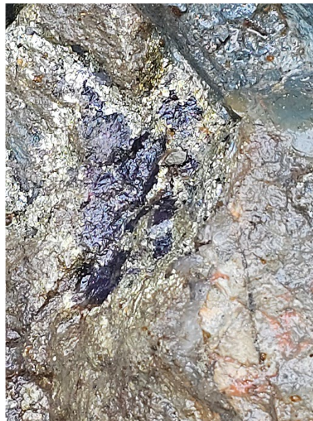
Figure 7: Chalcopryite-pyrite-pyrrhotite-covellite(?) massive sulphide vein at the Chevrier Prospect. Photo width 50cm. Estimated 70% sulphides within vein**.
