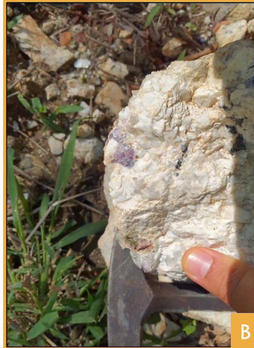
Photograph of sample BLR237 showing lepidolite minerals within pegmatite sample (Assay: 0.53% \text{Li}_2\text{O} )
