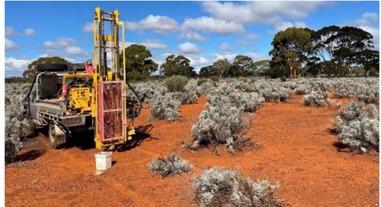
Auger rig used for calcrete sampling
