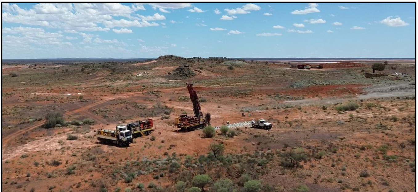
Figure 3. Topdrill RC rig at Baxter-Golconda testing for extensions to the high-grade gold mineralisation (December 2024).
