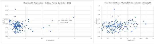
In fresh rock samples, a regression model for block density determination has been made by plotting assay interval Fe (%) + S (%) from the interval where the SG measurement was made against the SG measurement. Fe and S are the two elements that form pyrite which is the mineral that is commonly associated with gold and base metal mineralisation at Hualilan. SG plotted against (Fe+S) follows a linear trend within the mineralised domains for oxide and fresh rock as shown below.
