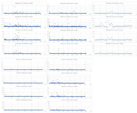
For GNDD001 – GNDD010 samples analysed by MSA in 2019, three different Certified Standard Reference pulp samples (CRM) with known values for Au Ag Pb Cu and Zn were submitted with samples of drill core to test the precision and accuracy of the analytic procedures MSA laboratory in Canada. 26 reference analyses were analysed in the samples submitted in 2019. The standards demonstrate suitable precision and accuracy of the
