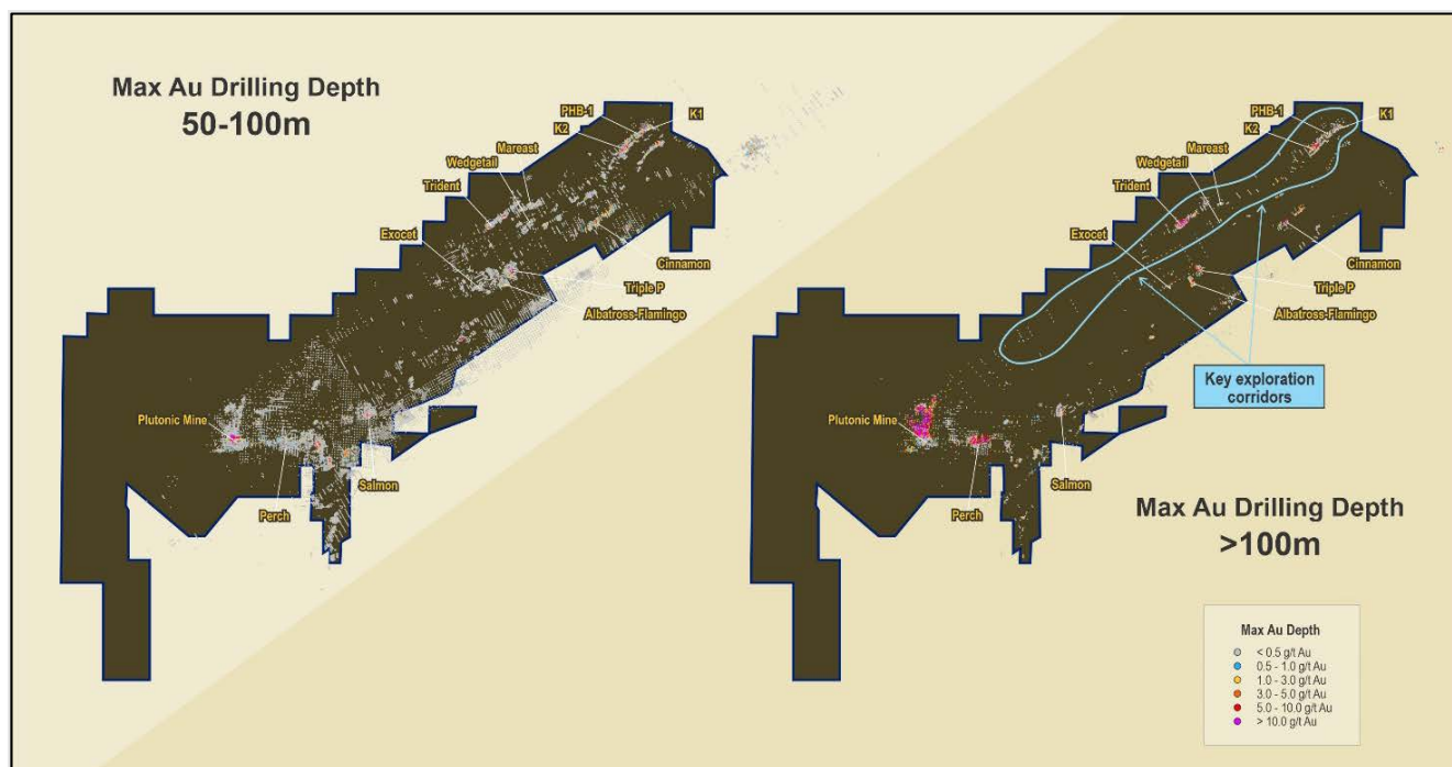
Figure 11: Plutonic gold belt showing mineralisation below 100m versus drilling density below 100m
