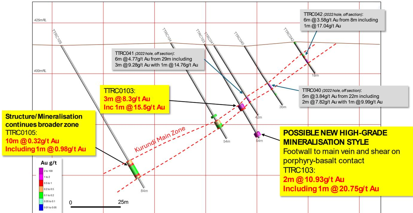
**Figure 4: Cross Section (oblique section, location shown in Figure 4) showing holes near to the new high grade mineralisation footwall to the Kurundi Central main zone, TTRC040-42 are 2022 holes off section.**
