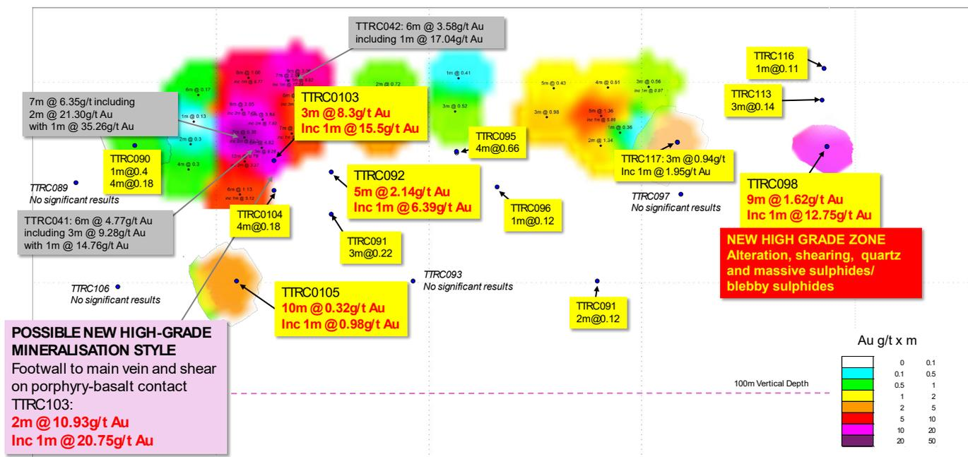
**Figure 3: Long projection of the Central Main Kurundi mineralized zone beneath the central workings area. View is perpendicular to the main vein which dips approximately 35° towards 215°. New results shown in yellow boxes, 2022 results shown in grey boxes, light purple box is for the footwall intersection.**
