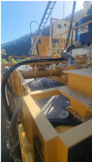
**Figure 7 Gravity circuit screen**
