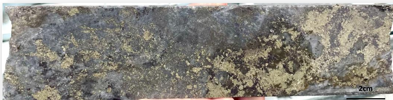
Figure 1: Core photo of polymetallic gold-copper mineralisation from 503.7m to 503.9m in ZRSD24166. Laboratory assays from this sample returned 1.0g/t Au, 0.5% Cu, 0.4% Pb, 1.1% Zn. Common mineralogy includes pyrite (light yellow), chalcopyrite (bright yellow), galena (grey), pyrrhotite (brassy/bronze) and sphalerite (dark brown/black).
