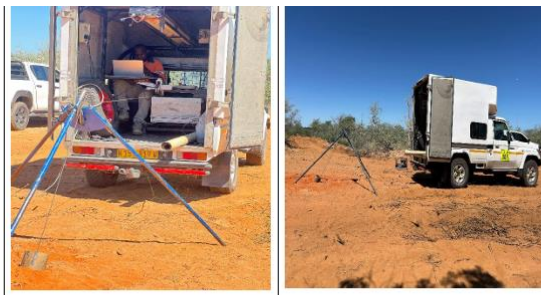
Figure 4: Optical Televiewer (OPTV) downhole logging underway at Fiesta.
