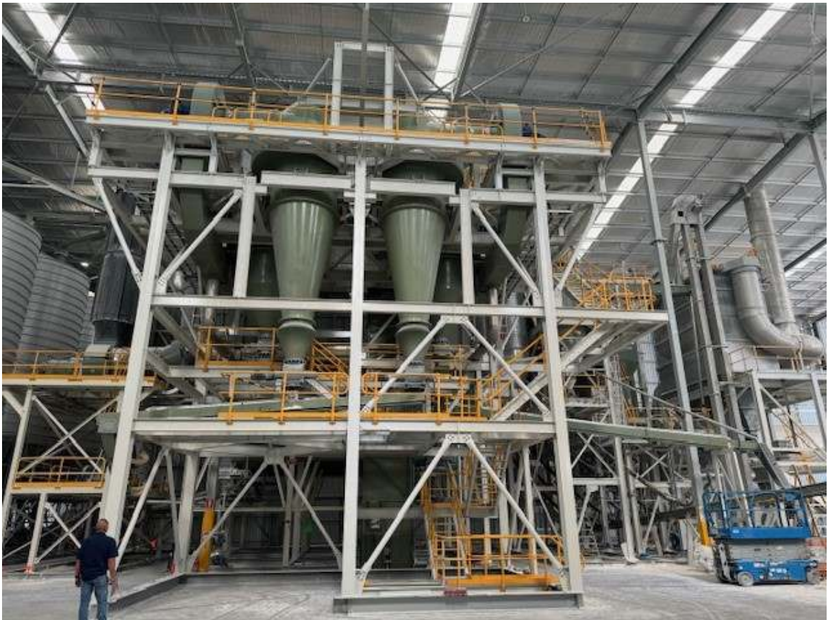
The new classifier plant fully installed and commissioned (12m x 11m x 18m high)
