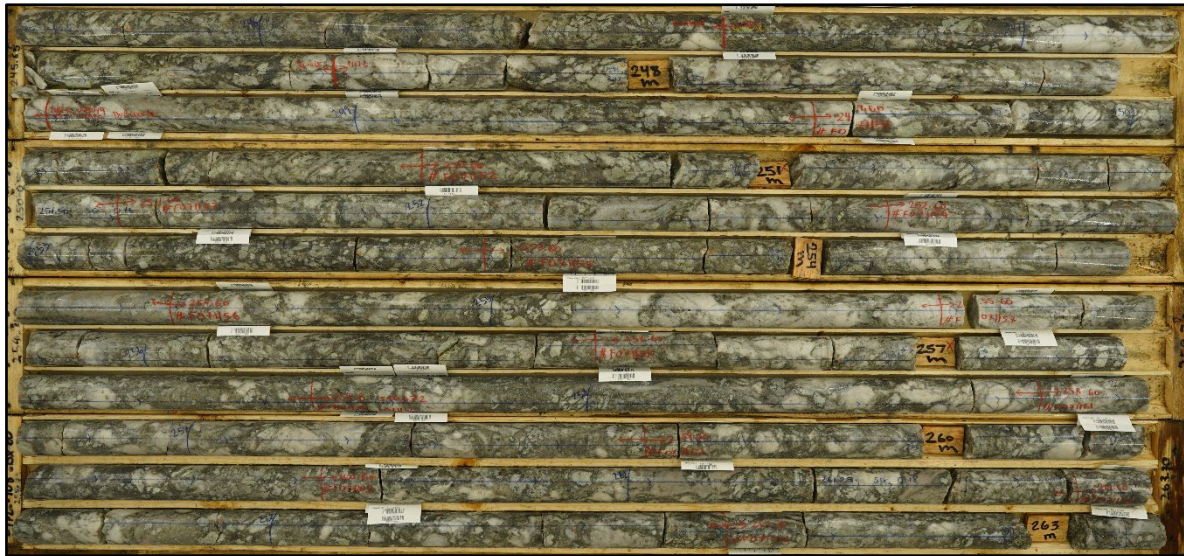
Figure 3 – Core box containing spodumene grading 1.47% Li 2 O in hole 24FL-108_245.65m-263.1m, Falcon Little Lake (refer to Appendix 1, Table 1, significant intercept table).
