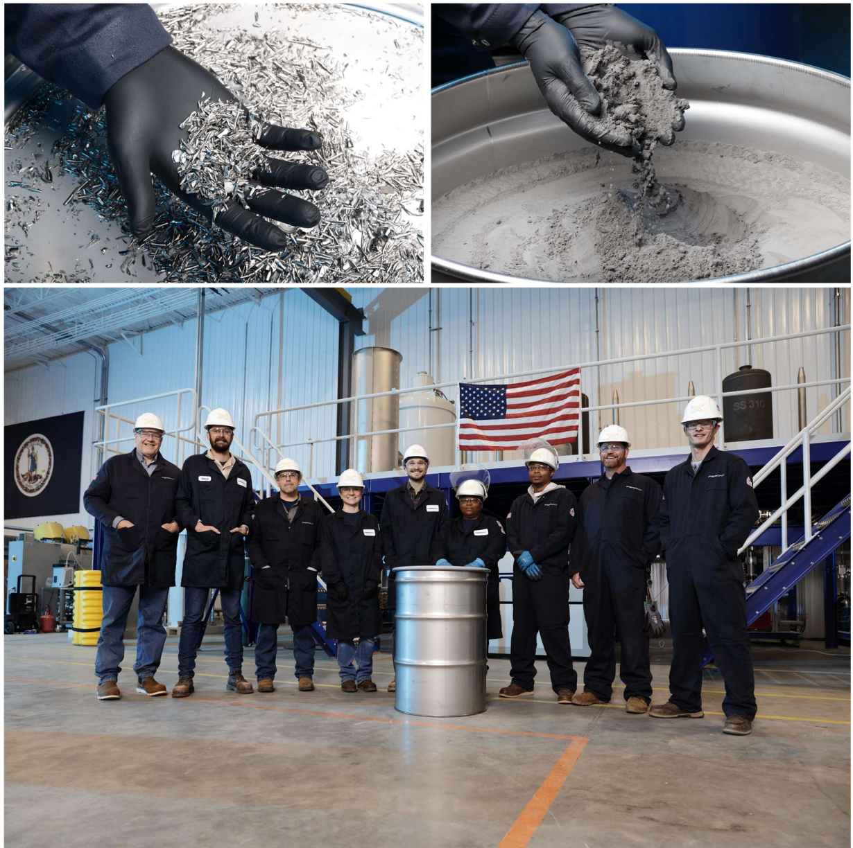
Figure 1 (clockwise from top left): Titanium scrap; Finished titanium metal powder; IperionX metal production team with a drum of finished titanium metal powder in front of the HAMR furnace at the Titanium Production Facility.
